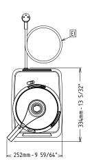
Electric Supply voltage: 220-240 V/1N ph/50/60 Hz **Electrical power max.:** 0.75 kW 0.75 kW **Total Watts:** Capacity: Performance (up to): Capacity: 3.6 litres Key Information: External dimensions, Width: 252 mm External dimensions, 334 mm Depth: External dimensions, Height: 476 mm 16.9 kg **Shipping weight:** Meat mincing capacity: 0 kg Mayonnaise preparation 0 kg capacity: Pastry preparation capacity: 0 kg
